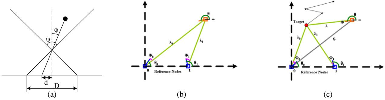
Fig. 1. (a) Pinhole camera model. (b) Localization using observations between nodes. (c) Localization using common observations of moving target.
