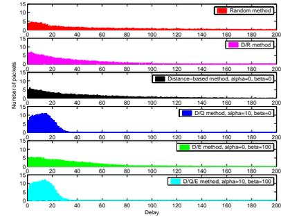
Fig. 8. Delay histograms for event data in distance-based schemes.
