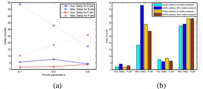
Fig. 9. (a) Effect of relative priority level  $p$  in the A/Q/E method. (b) Effects of 50% unlocalized nodes on the Ave. and Max. delays of event and periodic packets in the A/Q/E and D/Q/E methods.
