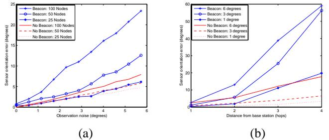
Fig. 2. (a) Effect of observation noise on sensor orientation error. (b) Effect of number of hops to base station on sensor orientation error in presence of observation noise.
