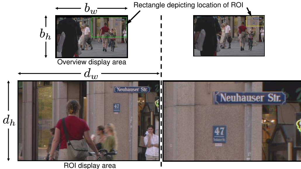
Figure 1: User interface: The display screen consists of the overview display area and the ROI display area. The effect of changing the zoom factor can be seen by comparing left and right hand sides of the figure.
